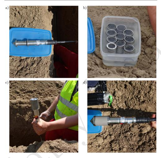
**Figure 3.** Installation of porometer: A – sensor prior to the installation of the filter, B – filters prior to the installation, C – filter installation, D – sensors after the installation of the filter [8].
