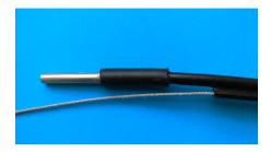
**Figure 14.** Final/ending sensor on a sensing cable with a security sealing cap. A steel wire is visible, which is later fastened to a leading cone during cable ground installation.
