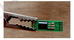
Figure 13. Intermediate sensors mounted along the cable with a dedicated PCB (printed circuit board)
