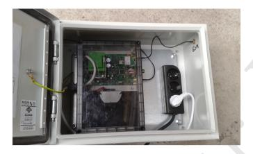
**Figure 18.** Edge Node with emergency power supply.
